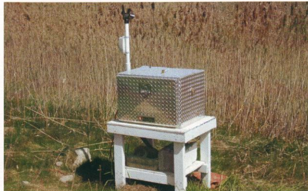
Hydrogen Sulfide monitor located downwind of landfill
